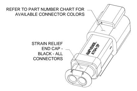
RECEP, 2 PIN, AT, STRAIN RELIEF, REDUCED DIA WIRE SEAL
