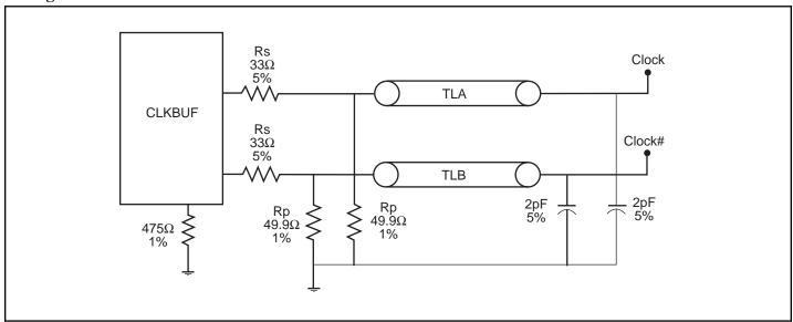
Figure 2. Configuration test load board termination
