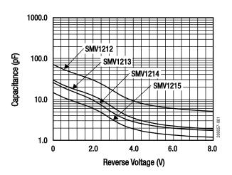
Figure 1. Capacitance vs Reverse Voltage
