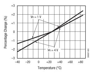
Figure 3. Relative Capacitance Change vs Temperature
