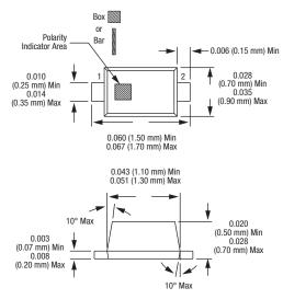
Dimensions are in inches (millimeters shown in parentheses) 200057-006
