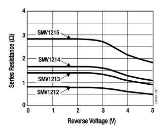
Figure 2. Series Resistance vs Reverse Voltage @ 500 MHz
