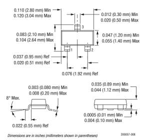
Figure 8. SOT-23 Package Dimensions
