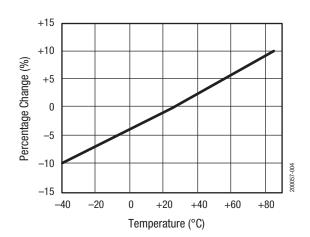
Figure 4. Relative Series Resistance Change vs Temperature @ 500 MHz
