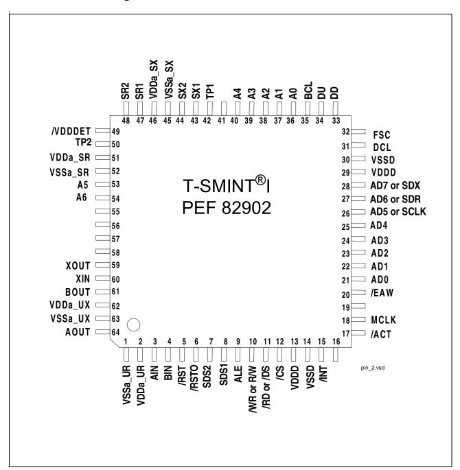
Figure 1 Pin Configuration
