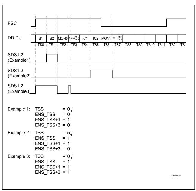
Figure 19 Data Strobe Signal Generation
