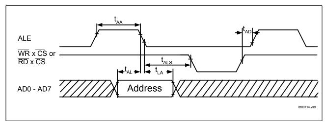
Figure 67 Multiplexed Address Timing
