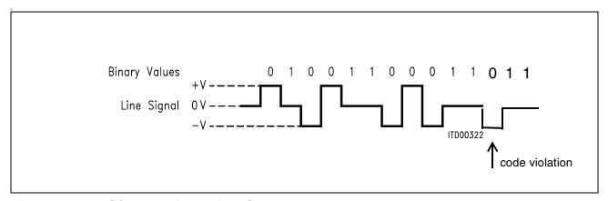
Figure 37 S/T -Interface Line Code
