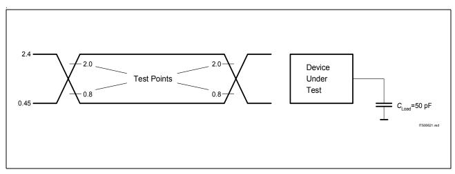
Figure 61 Input/Output Waveform for AC Tests
