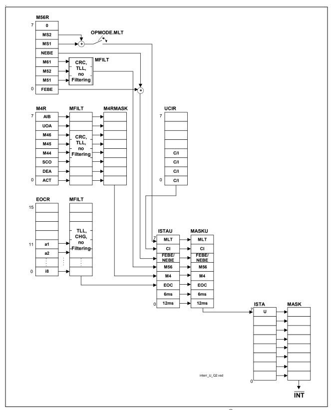
Figure 77 Interrupt Structure U-Transceiver Q-SMINT®I: 2B1Q
