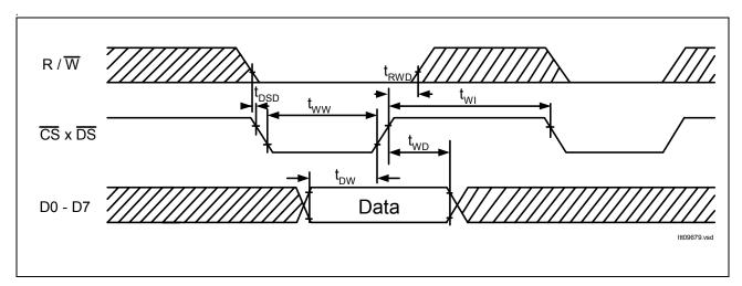
Figure 70 Microprocessor Write Cycle
