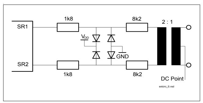
Figure 56 External Circuitry S-Interface Receiver
