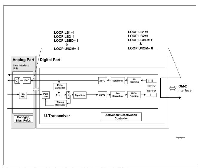
Figure 52 Loopbacks Featured by Register LOOP
