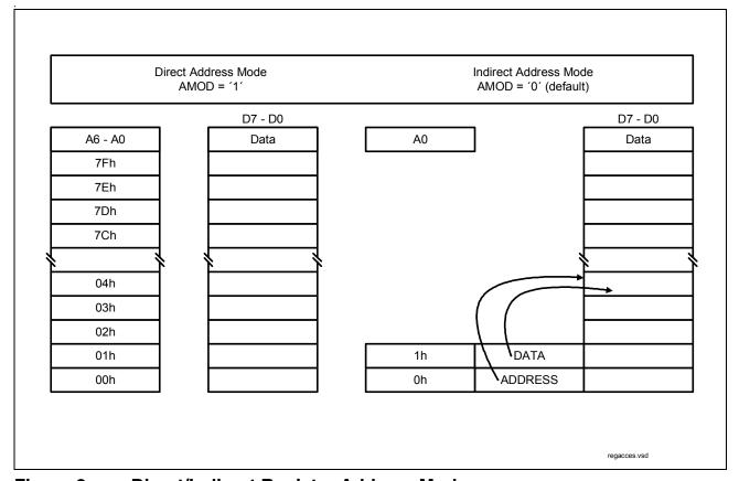
Figure 8 Direct/Indirect Register Address Mode
