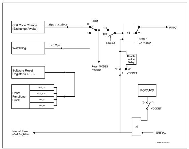
Figure 9 Reset Generation of the T-SMINT®I<sup>1)</sup>
