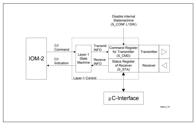
Figure 39 S-Transceiver Control
