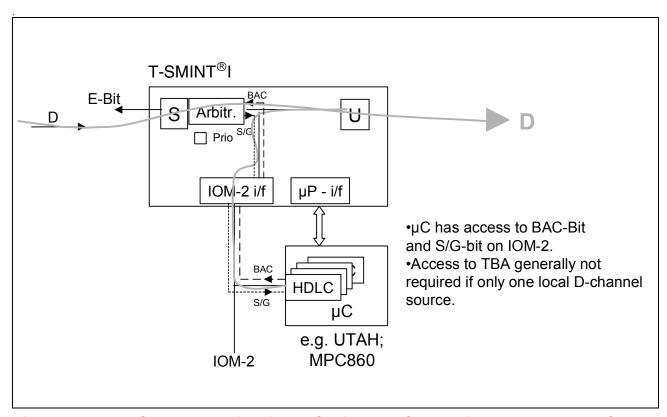
Figure 26 D-Channel Arbitration: μC with HDLC and Direct Access to TIC Bus
