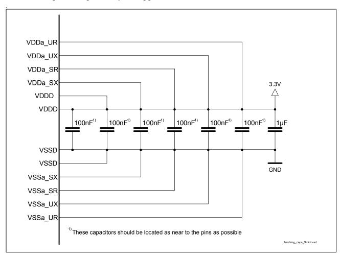
Figure 53 Power Supply Blocking
