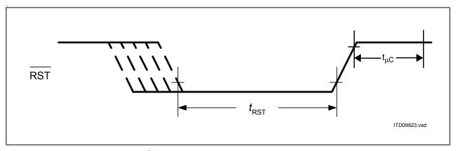
Figure 72 Reset Input Signal
