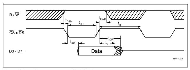
Figure 69 Microprocessor Read Timing
