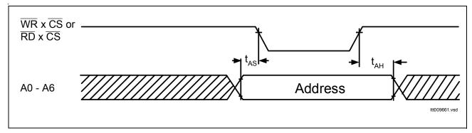
Figure 68 Non-Multiplexed Address Timing
