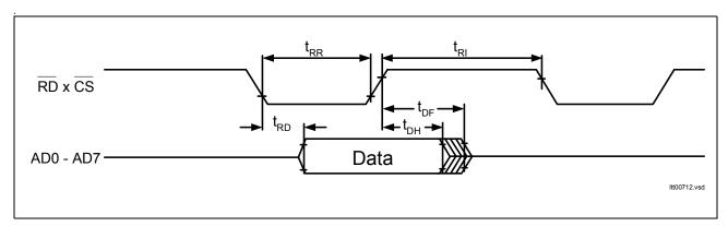
Figure 65 Microprocessor Read Cycle
