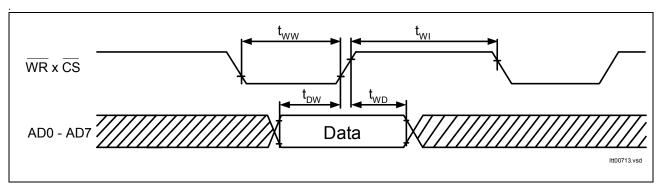
Figure 66 Microprocessor Write Cycle
