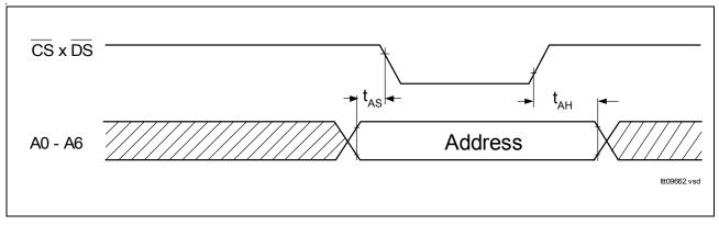
Figure 71 Non-Multiplexed Address Timing
