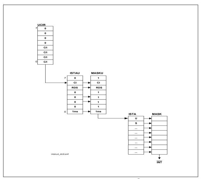
Figure 78 Interrupt Structure U-Transceiver T-SMINT®I: 4B3T
