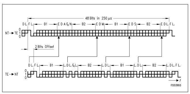
Figure 38 Frame Structure at Reference Points S and T (ITU I.430)
