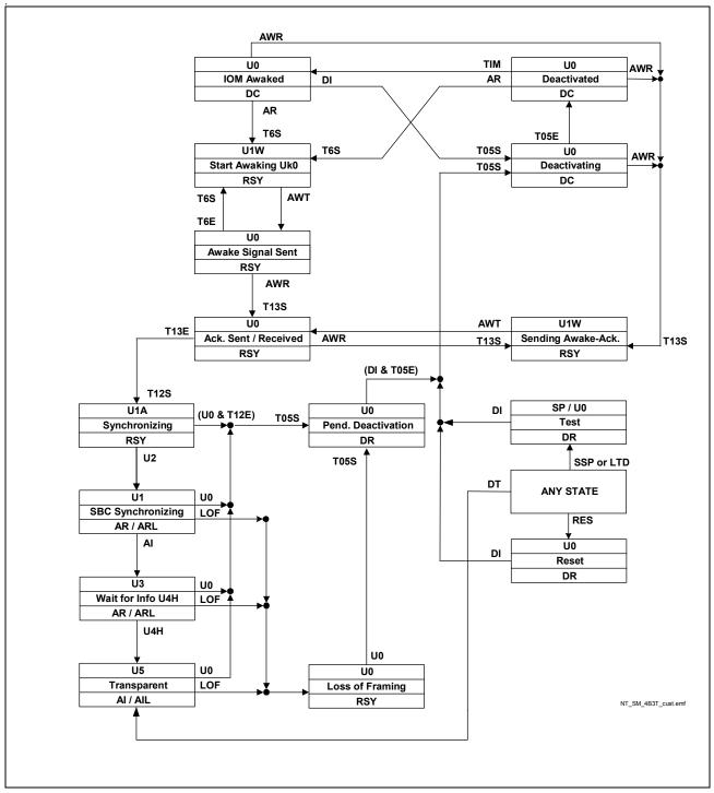
Figure 76 IEC-T/NTC-T Compatible State Machine T-SMINT®I: 4B3T
