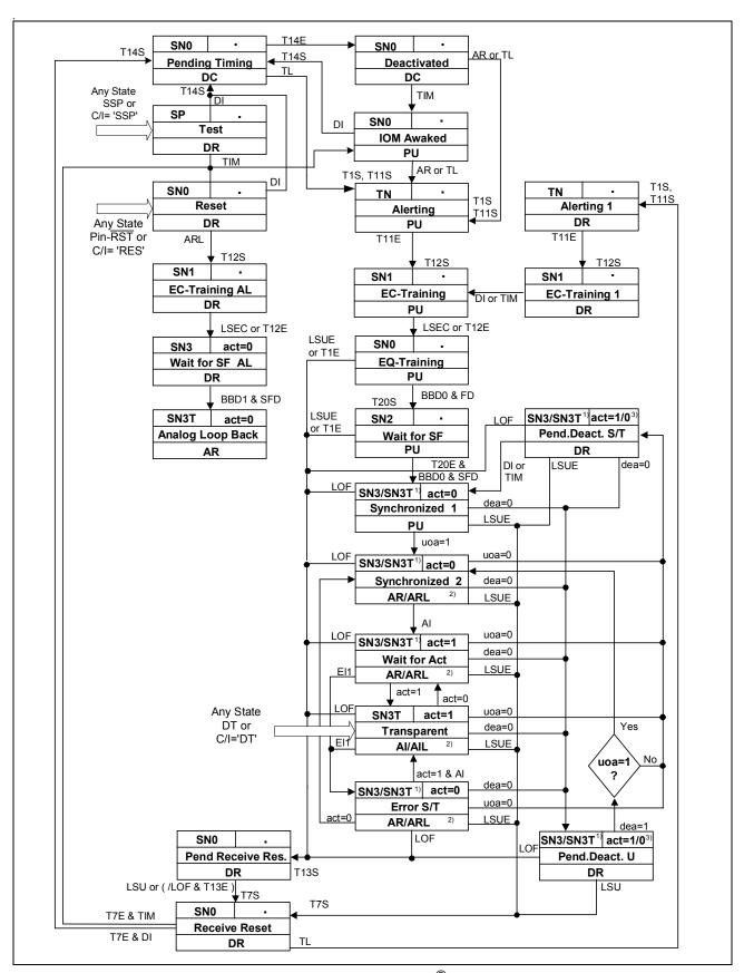
Figure 75 Simplified State Machine Q-SMINT®I: 2B1Q
