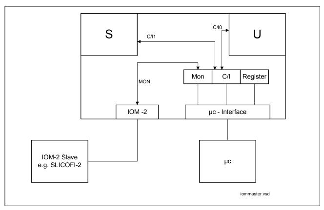
Figure 4 Control via µP Interface
