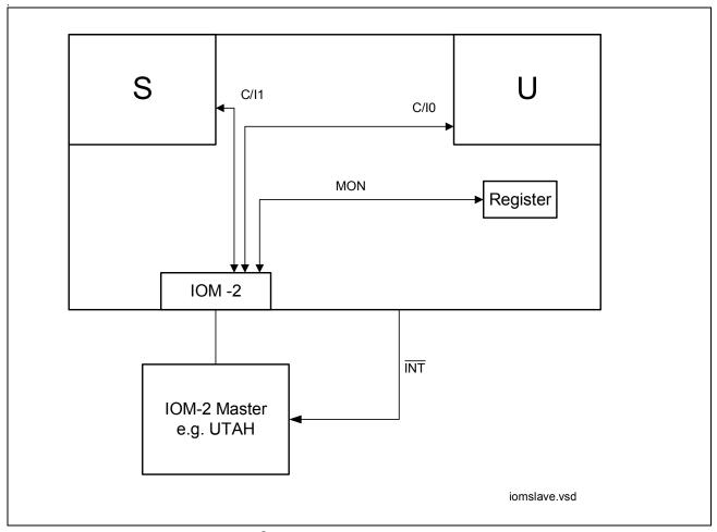
Figure 5 Control via IOM®-2 Interface
