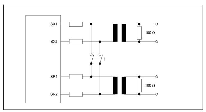
Figure 50 External Loop at the S/T-Interface
