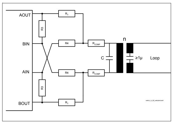
Figure 54 External Circuitry U-Transceiver with External Hybrid
