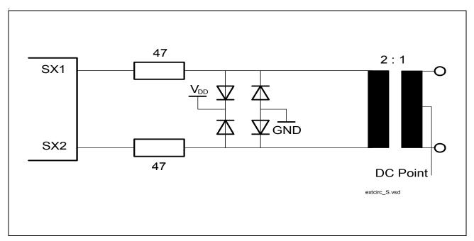
Figure 55 External Circuitry S-Interface Transmitter
