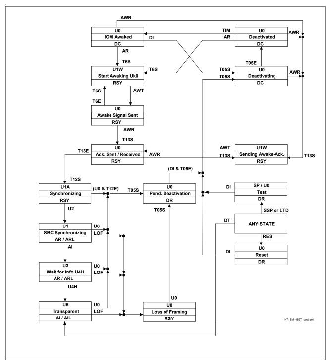
Figure 35 NT State Machine (IEC-T/NTC-T Compatible)
