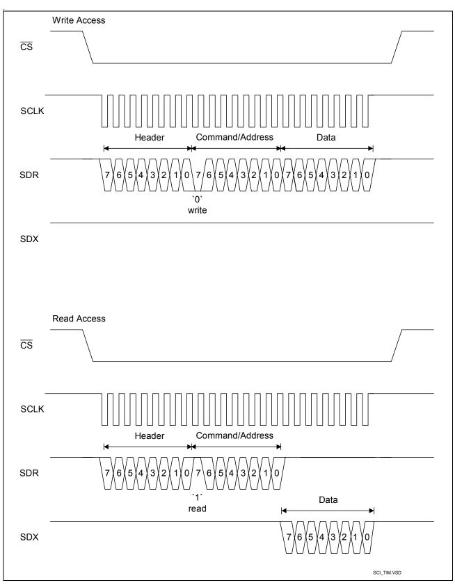
Figure 6 Serial Control Interface Timing
