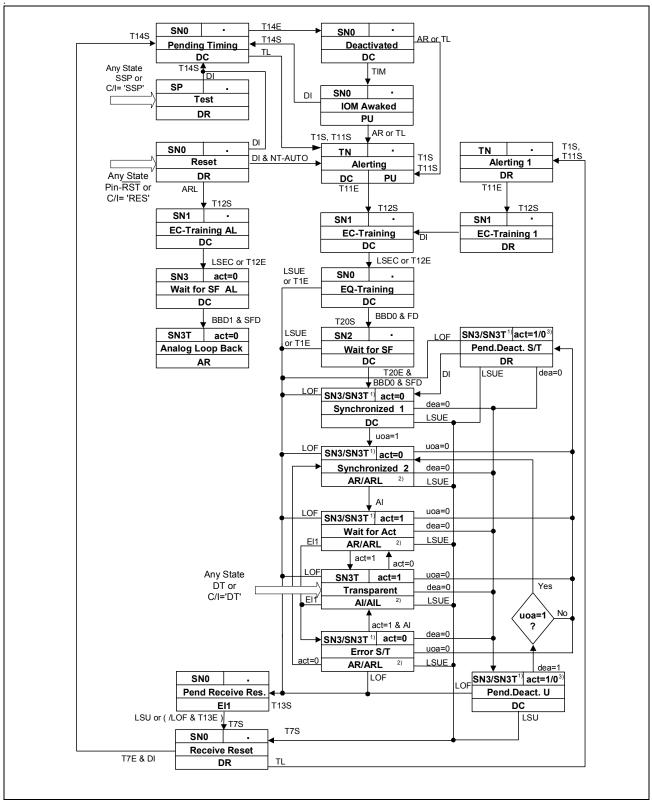
Figure 74 NTC-Q Compatible State Machine Q-SMINT®I: 2B1Q
