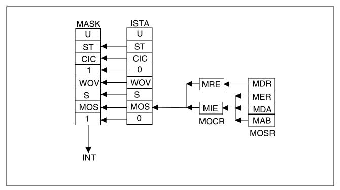
Figure 24 MONITOR Interrupt Structure
