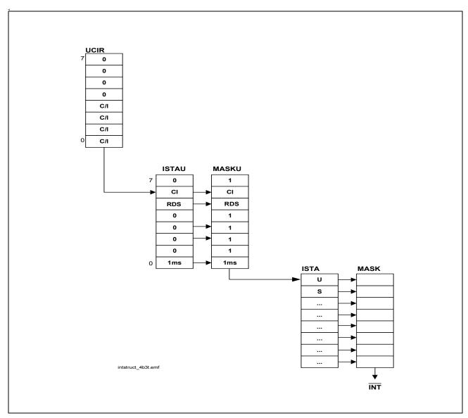
Figure 36 Interrupt Structure U-Transceiver
