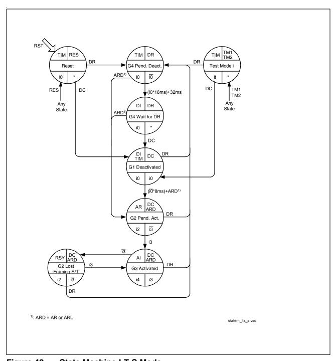
Figure 42 State Machine LT-S Mode
