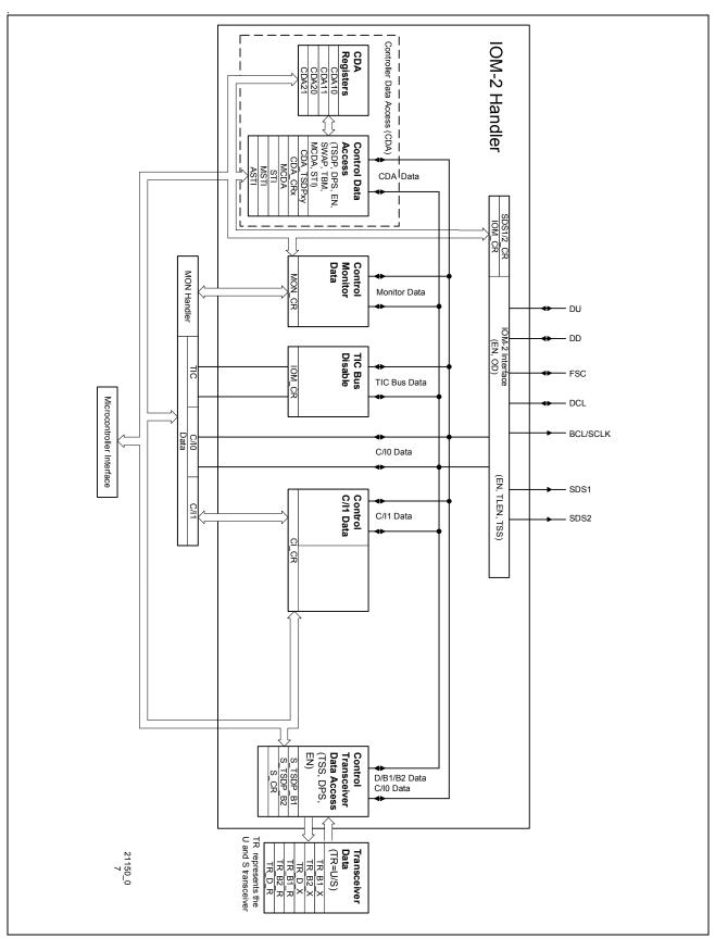
Figure 11 Architecture of the IOM®-2 Handler
