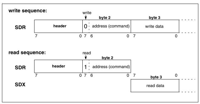
Figure 7 Serial Command Structure
