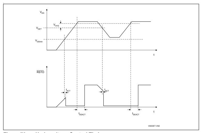
Figure 73 Undervoltage Control Timing
