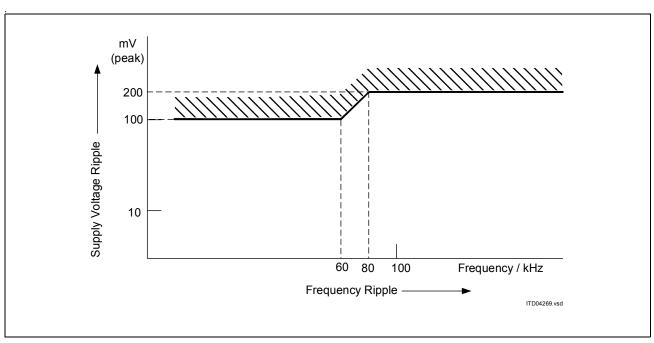
Figure 60 Maximum Sinusoidal Ripple on Supply Voltage
