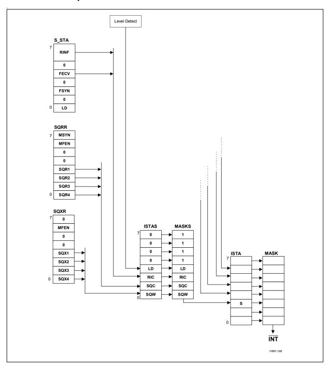
Figure 43 Interrupt Structure S-Transceiver
