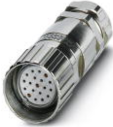
M23 socket, 19-pos., straight, freely configurable, with solder connection, for external cable diameter of 10 mm ... 14 mm
