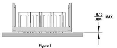
There should be no broken stand-offs along the perimeter of the part (an indication of over-pressing).
