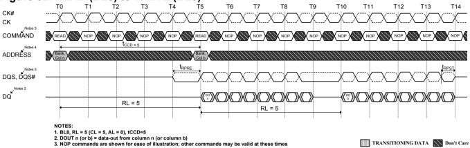
4. BL8 setting activated by either MR0[A1:0 = 00] or MR0[A1:0 = 01] and A12 = 1 during READ commands at T0 and T4 5. DQS-DQS# is held logic low at T9
