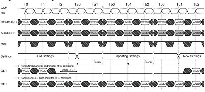
Figure 6. tMRD timing
