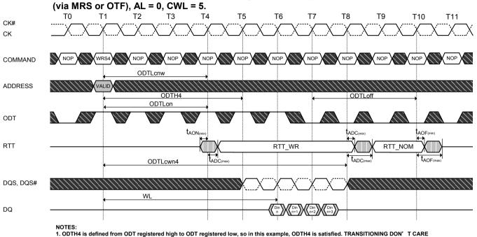
1. ODTH4 is defined from ODT registered high to ODT registered low, so in this example, ODTH4 is satisfied. TRANSITIONING DON' 2. ODT registered low at T5 would also be legal.
