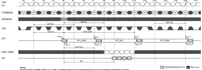
NOTES: Example for BC4 (via MRS or OTF), AL = 0, CWL = 5. ODTH4 applies to first registering ODT high and to the registration of the Write com In this example, ODTH4 would be satisfied if ODT went low at T8 (4 clocks after the Write command).
