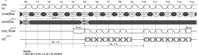
DOUT n (or b) = data-out from column n (or column b)
