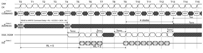
NOTES: 1. BC4, RL = 5 (CL = 5, AL = 0), WL = 5 (CWL = 5, AL = 0) 2. DOUT n = data-out from column, DIN b = data-in from column b. 3. NOP commands are shown for ease of illustration; other commands may be valid at these times. 4. BC4 setting activated by MR0[A1:0 = 01] and A12 = 0 during READ command at T0 and WRITE command at T4.
