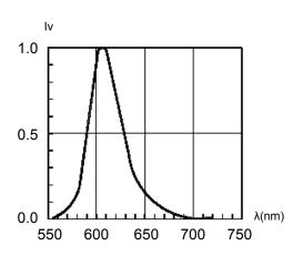
Fig. 1 Relative Luminous Intensity vs. Wavelength
