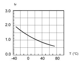
Fig. 3 Relative Luminous Intensity vs. Temperature
