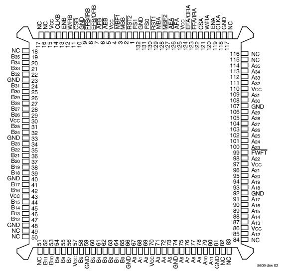
Electrical pin 1 in center of beveled edge. Pin 1 identifier in corner.
