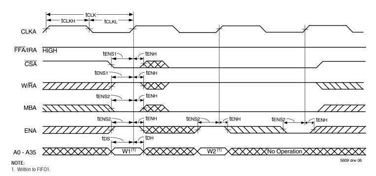
Figure 4. Port A Write Cycle Timing for FIFO1 (IDT Standard and FWFT Modes)
