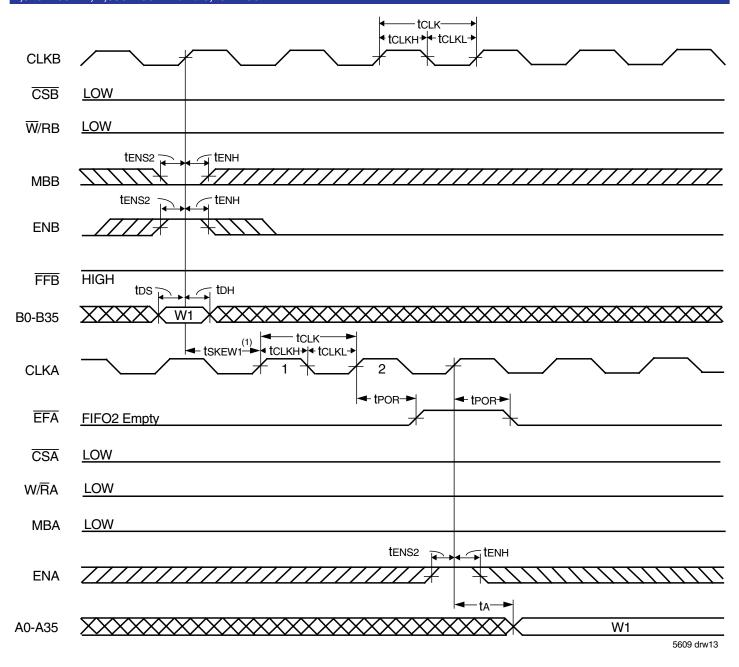
1. tskew1 is the minimum time between a rising CLKB edge and a rising CLKA edge for EFA to transition HIGH in the next CLKA cycle. If the time between the rising CLKB edge and rising CLKA edge is less than tskew1, then the transition of EFA HIGH may occur one CLKA cycle later than shown.
