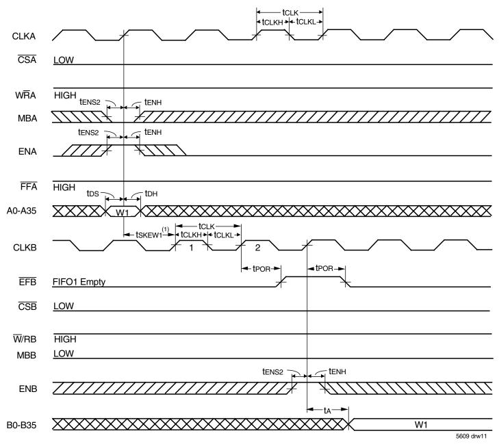
1. tskew1 is the minimum time between a rising CLKA edge and a rising CLKB edge for EFB to transition HIGH in the next CLKB cycle. If the time between the rising CLKA edge and rising CLKB edge is less than tskew1, then the transition of EFB HIGH may occur one CLKB cycle later than shown.
