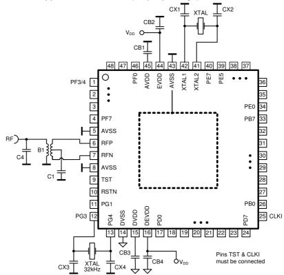
The power supply bypass capacitors (CB2, CB4) are connected to the external analog supply pin (EVDD, pin 44) and external digital supply pin (DEVDD, pin 16). The capacitor C1 provides the required AC coupling of RFN/RFP.
