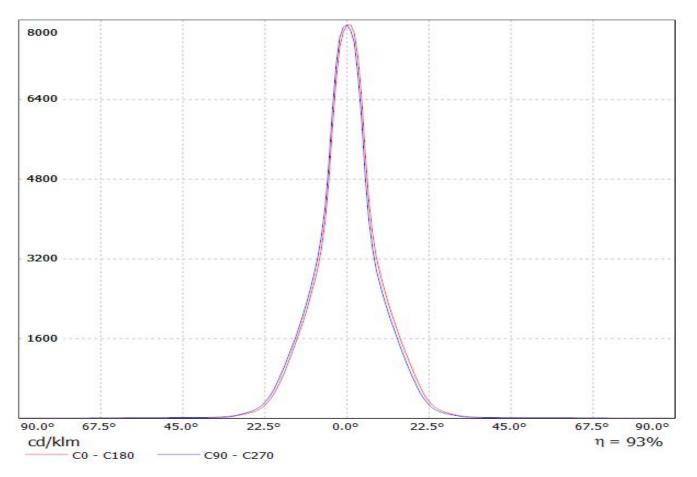
Luminaire: LEDil Oy FA11937\_LXM\_RS Lamps: 1 x Cree XM-L (100Im@250mA) XMLAWT-00-0000-0000T6051 P=0.7W I=250mA
