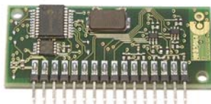
Figure 13: Receiver devices RCM 110 and RCM 120
