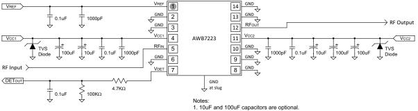
2. Applications that have large supply voltage transients may benefit from the use of TVS diodes. For such applications, recommended TVS diodes are SM05T1G or SMJ5.0A.
