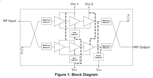
AWB7223 1.930 -1.995 GHz Small-Cell Power Amplifier Module Data Sheet
