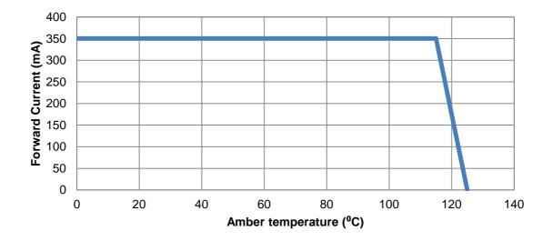
Fig 8. Forward Current Degrading Curve of LTPL-P05EXXXX
