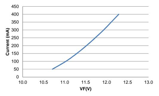
Fig 6. Forward Current vs. Forward Voltage of LTPL-P05EXXXX
