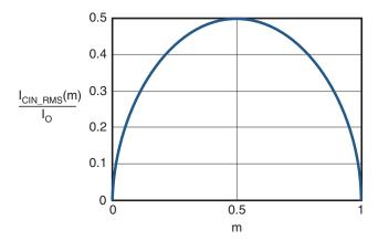
Figure 2. ICIN vs. Voltage Conversion Ratio
