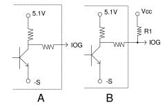
Figure 23 The application of IOG
