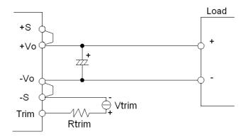
Figure 20 Trimmed by V<sub>trim</sub> circuit
