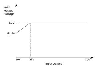
Figure 19 Trim-up-able voltage vs. input voltage
