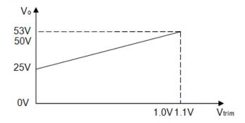
Figure 21 V<sub>trim</sub> voltage vs. output voltage (R<sub>trim</sub>=5.97k)
