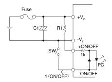
Figure 16 Connection of remote ON/OFF control (A)
