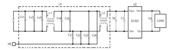
Figure 11 EMC test configuration
