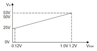
Figure 22  $V_{trim}$  voltage vs. output voltage ( $R_{trim}$ =5.1k $\Omega$ )
