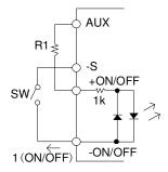
Figure 17 Connection of remote ON/OFF control (B)
