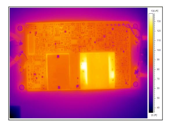
Figure 14 Thermal image,  $48V_{\rm in}$ ,  $48V_{\rm o}$ , full load, room temperature
