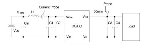
Figure 24 Input ripple & output ripple & noise test configuration
