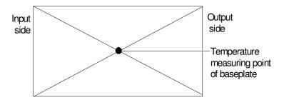
Figure 12 Temperature test point on baseplate
