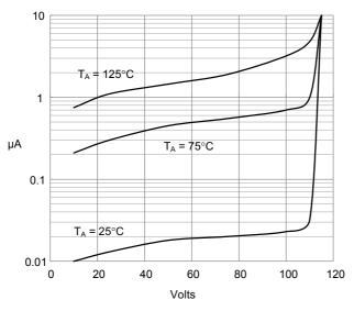
Instantaneous Reverse Current - Micro Amps*versus* Percent Of Rated Peak Reverse Voltage - Volts
