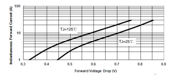
Fig.3-Typical Instantaneous Forward Voltage Characteristics
