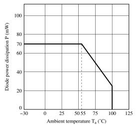
Fig.4 Total Power Dissipation vs. Ambient Temperature
