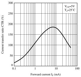
Fig.9 Relative Current Transfer Ratio vs.
