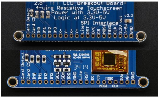
Don't forget, we're using the SPI interface side of the PCB!
