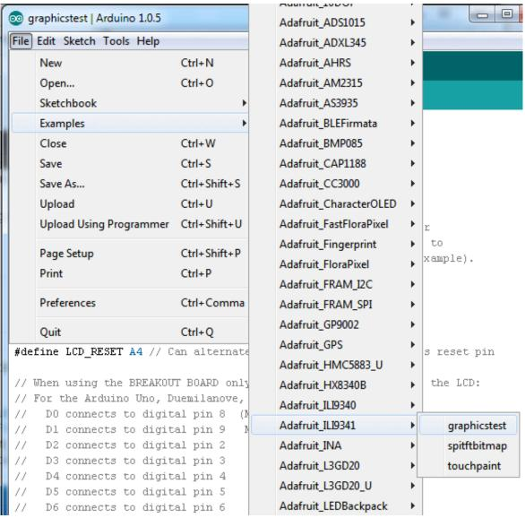
After restarting the Arduino software, you should see a new **example** folder called **Adafruit\_ILI9341** and inside, an example called **graphicstest**. Upload that sketch to your Arduino. You may need to press the Reset button to reset the arduino and TFT. You should see a collection of graphical tests draw out on the TFT.
