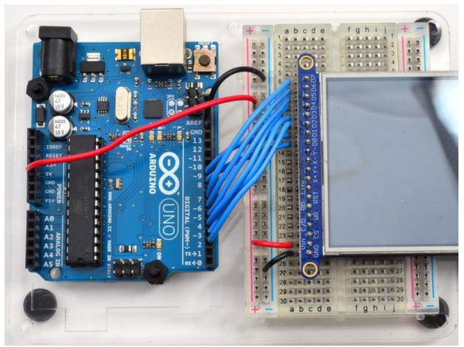
Now you can connect the remaining 6 pins over. Connect **D2-D7** on the TFT pins to digital **2** thru **7** in that order. If you're using a Mega, connect the TFT Data Pins **D2-D7** to Mega pins **#24-29**, in that order. Those Mega pins are on the 'double' header.
