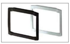
**F0:** The F0 frame is used for edge covering of a continuous front panel (FP). Mounting on the base is by clipping-on and pressing tight. In connection with base and front panel: protection class IP 40.
