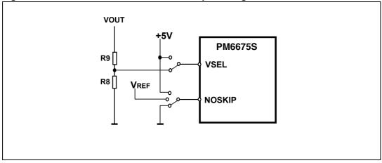
The PM6675S has been designed to satisfy the widest range of applications. The device is provided with some multilevel pins which allow the user to choose the appropriate configuration. The VSEL pin is used to firstly decide between fixed preset or adjustable (user defined) output voltages.
