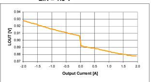
Figure 9. VOUT line regulation, 1.5 V, 0 A
