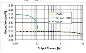
Figure 8. LOUT load regulation, LOUT = 0.9 V, LIN = 1.5 V
