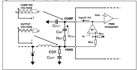
Figure 35. Circuitry for output ripple compensation
