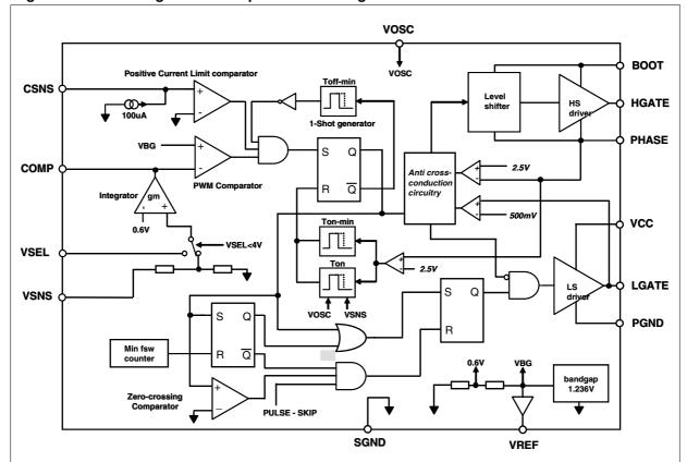
Figure 34. Switching section simplified block diagram
