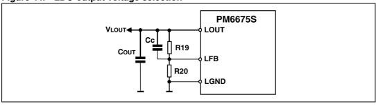
A compensation capacitor Cc must be added to adjust the dynamic response of the loop. The value of Cc is calculated according to the desired bandwidth of the LDO regulator and depends on the value of the feedback resistors. In most of applications the pole due to the compensation capacitor is placed at 100-200 kHz (equation 24).
