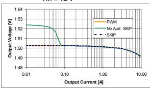
Figure 6. VOUT load regulation, 1.25 V, Vin = 12 V
