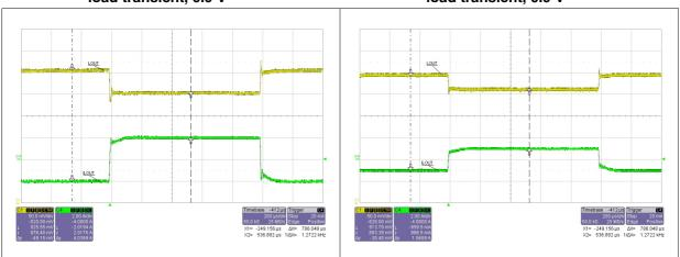
Figure 25. 0 A to 8 A VOUT load transient, PWM
