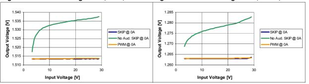
Figure 11. VOUT line regulation, 1.5 V
