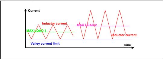
As the valley threshold is fixed, the greater the current ripple, the greater the DC output current will be. If an output current limit greater than  $I_{LOAD}(max)$  over all the input voltage range is required, the minimum current ripple must be considered in the previous formula.
