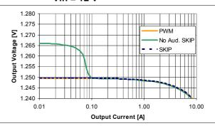
Figure 7. VOUT load regulation, 2.5 V, Vin = 12 V
