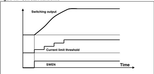
After a fixed 3ms total time, the soft-start finishes and UVP is released: if the output voltage doesn't reach the under voltage threshold within soft-start duration, the UVP condition is detected and the device performs a soft-end and latches off. Depending on the load conditions, the inductor current may or may not reach the nominal value of the current limit during the soft-start (*Figure 42* shows two examples).
