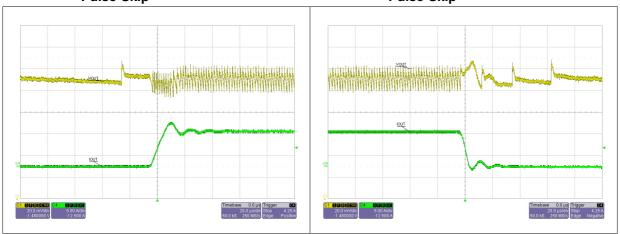
Figure 29. Over-voltage protection, VOUT = 1.5 V
