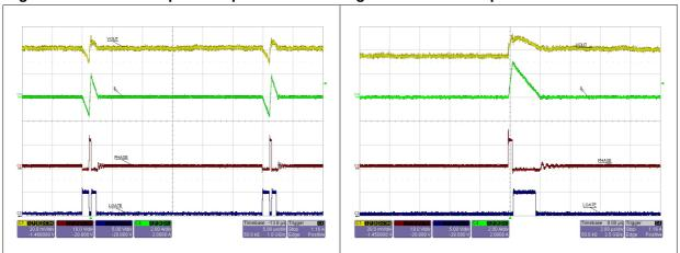
Figure 19. Power-up sequence VCC above UVLO
