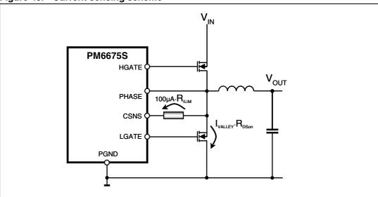
An internal 100  $\mu$ A current source is connected to  $C_{SNS}$  pin that is also the non-inverting input of the positive current limit comparator. When the voltage drop developed across the sensing parameter equals the voltage drop across the programming resistor  $R_{ILIM}$ , the controller skips subsequent cycles until the overcurrent condition is detected or the output UV protection latches off the device (see *Section 7.1.11: Switching section OV and UV protections on page 34*).
