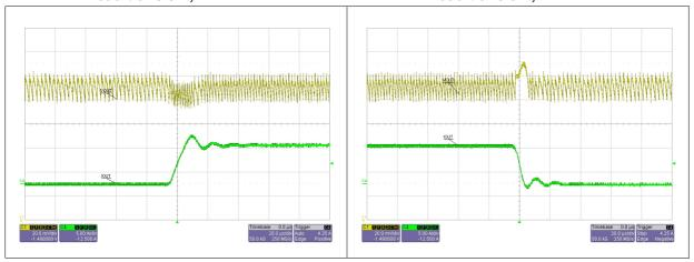
Figure 27. 0 A to 5 A VOUT load transient, Pulse-Skip
