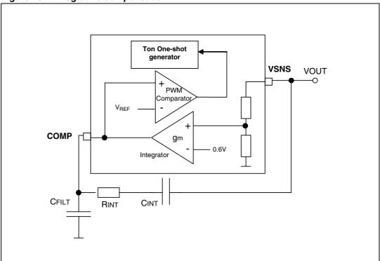
The stability of the system firstly depends on the output capacitor zero frequency. It must be verified that:
