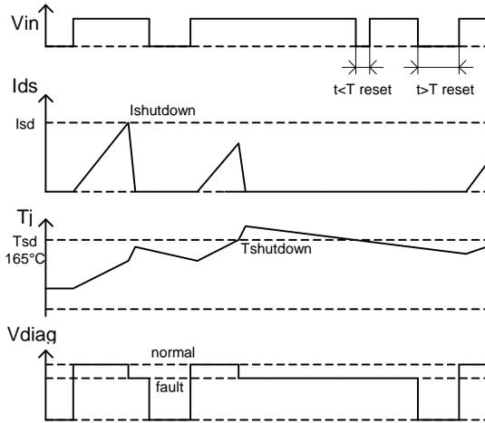
Figure 1 – Timing diagram
