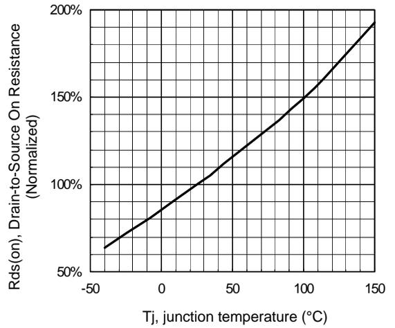
**Figure 6 - Normalized Rds(on) (%) Vs T<sub>j</sub> (°C)**
