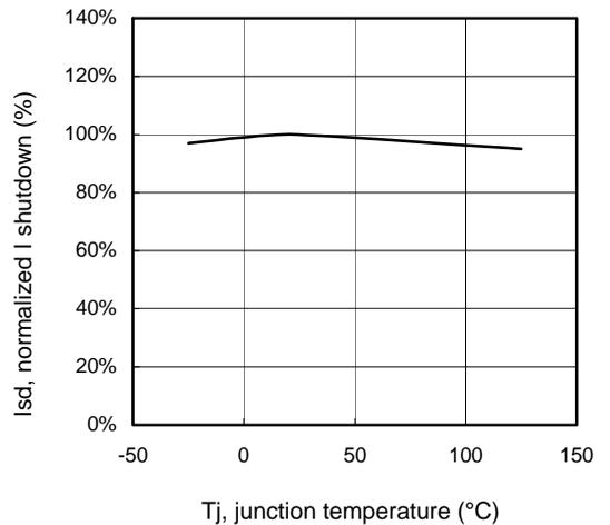
**Figure 8 – Normalized I shutdown (%) Vs junction temperature (°C)**
