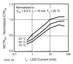
Fig. 8 - Normalized CTRcb vs. LED Current and Temperature
