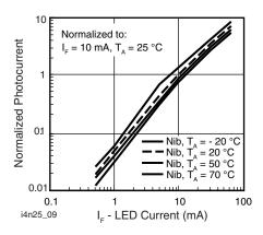
Fig. 9 - Normalized Photocurrent vs.  ${\rm I}_{\rm F}$  and Temperature
