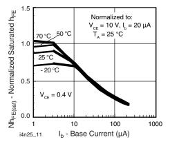
Fig. 11 - Normalized h<sub>FE</sub> vs. Base Current and Temperature
