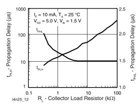
Fig. 12 - Propagation Delay vs. Collector Load Resistor
