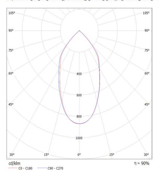
NOTE: The typical divergence will be changed by different color, chip size and chip position tolerance. The typical total divergence is the full angle measured where the luminous intensity is half of the peak value.
