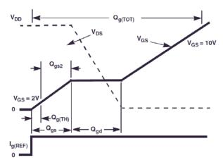
Figure 18. Gate Charge Waveforms
