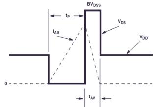
Figure 16. Unclamped Energy Waveforms
