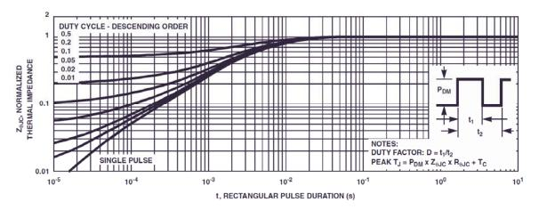
Figure 3. Normalized Maximum Transient Thermal Impedance
