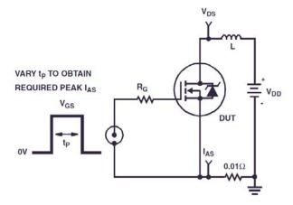
Figure 15. Unclamped Energy Test Circuit
