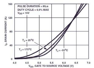
Figure 7. Transfer Characteristics
