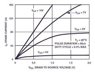
Figure 8. Saturation Characteristics
