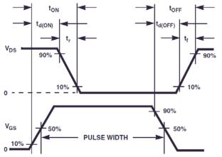
Figure 20. Switching Time Waveforms
