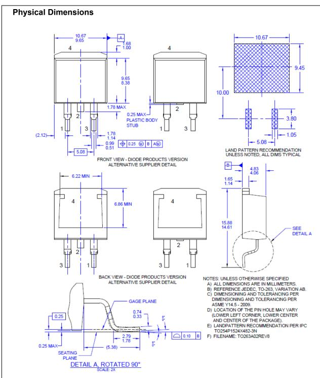
Figure 22. TO-263 2L (D2PAK), 4.445 x 10.16 x 15.24mm, TAPE REEL
