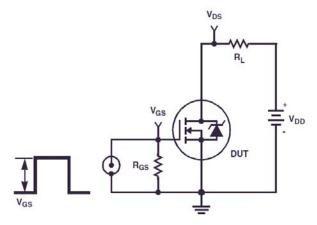
Figure 19. Switching Time Test Circuit
