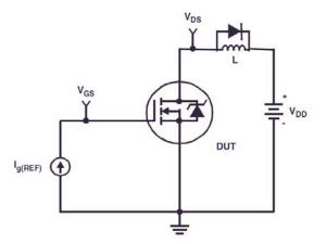
Figure 17. Gate Charge Test Circuit
