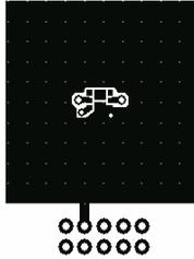
a)  $60^\circ\text{C/W}$  when mounted on a  $1\text{ in}^2$  pad of 2 oz copper
