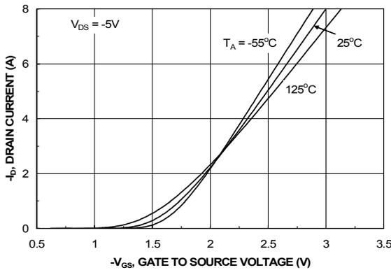
Figure 5. Transfer Characteristics
