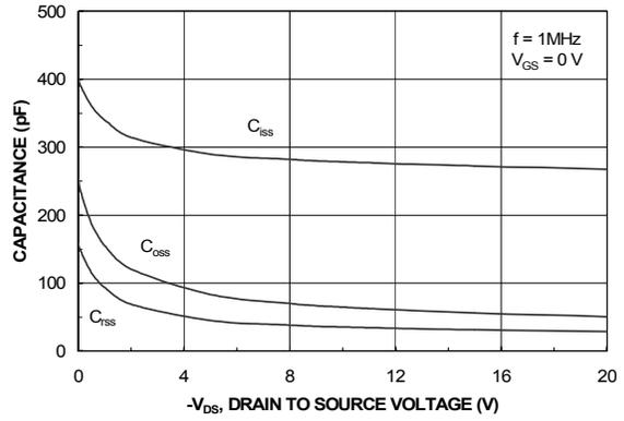
**Figure 8. Capacitance Characteristics**
