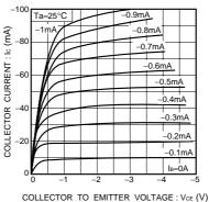
Fig.2 Grounded emitter output characteristics (I)
