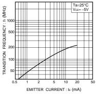
Fig.8 Gain bandwidth product vs. emitter current
