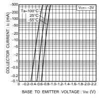
Fig.1 Grounded emitter propagation characteristics
