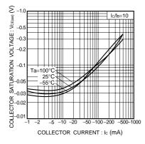
Fig.7 Collector-emitter saturation voltage vs. collector current (II)
