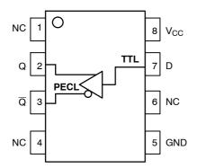
Figure 1. 8-Lead Pinout (Top View) and Logic Diagram
