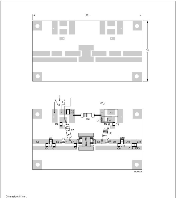
The components are situated on one side of the copper-clad printed-circuit board, the other side is unetched and serves as a ground plane. Earth connections from the component side to the ground plane are made by through metallization.
