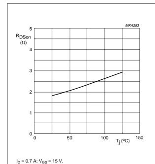
Fig.5 Drain-source on-state resistance as a function of junction temperature; typical values.
