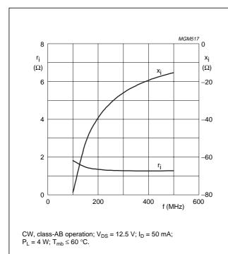
Fig.12 Input impedance as a function of frequency (series components); typical values.
