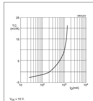
Fig.3 Temperature coefficient of gate-source voltage as a function of drain current; typical values.
