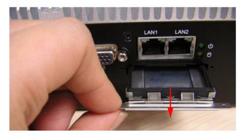
3. Remove the dummy CFast bracket.
