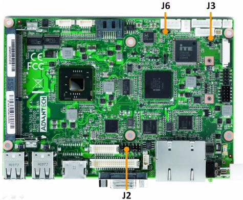
Figure 2.1 Jumper layout (Component Side)
