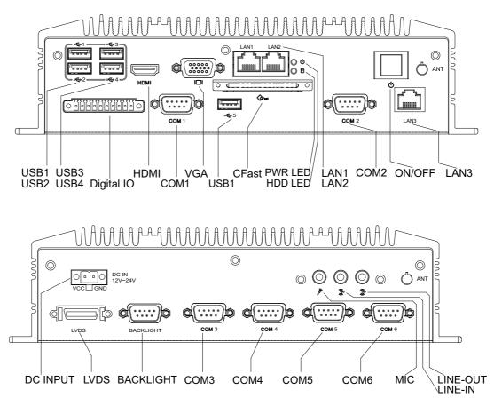
Figure 2.4 ARK-2120F IO connectors drawing
