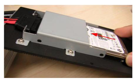
3. Screw the four screws on the side of HDD bracket. The screws are used to fix the HDD on the bracket. (The screws are in the accessory box.)
