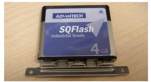
5. Push the CF tray back and secure with screws.
