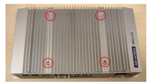
2. Unscrew the four screws on the right and left side of top cover
