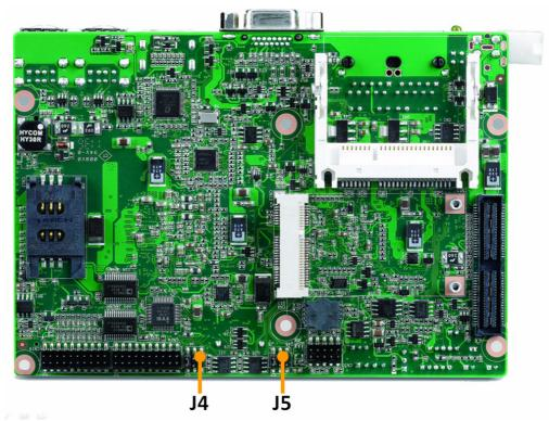
Figure 2.2 Jumper layout (Solder Side)
