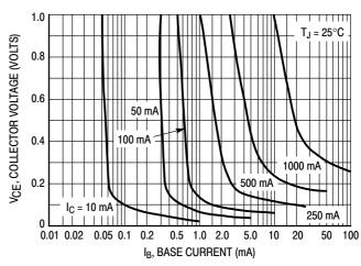
Figure 2. Collector Saturation Region
