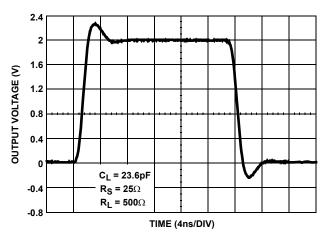
FIGURE 20. LARGE SIGNAL TRANSIENT RESPONSE
