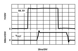
FIGURE 16. CHANNEL TO CHANNEL TRANSIENT RESPONSE  $V_{\mbox{\scriptsize IN}}$  = 1V, R<sub>S</sub> = 25, C<sub>L</sub> = 23.6pF
