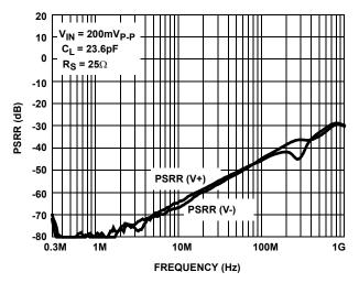
FIGURE 9. PSRR CHANNELS
