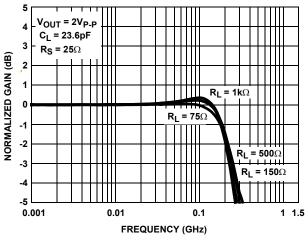
FIGURE 4. LARGE SIGNAL GAIN vs FREQUENCY vs RL
