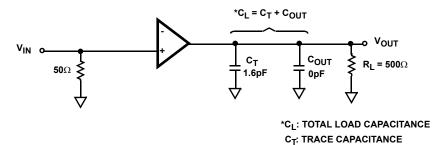
FIGURE 24A. SMALL SIGNAL 200mV<sub>P-P</sub> APPLICATION CIRCUIT
