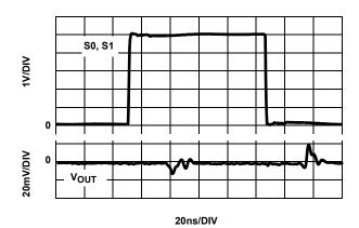
FIGURE 15. CHANNEL TO CHANNEL SWITCHING GLITCH  $V_{IN} = 0 V,\, R_S = 25,\, C_L = 23.6 pF$
