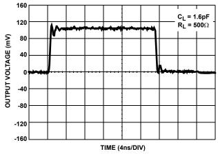
FIGURE 19. SMALL SIGNAL TRANSIENT RESPONSE
