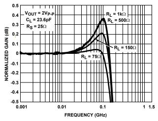
FIGURE 8. LARGE SIGNAL 0.1dB GAIN vs FREQUENCY vs RI
