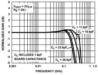
FIGURE 3. LARGE SIGNAL GAIN vs FREQUENCY vs CL
