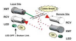
Product with FiberAlert enabled —Remote Site stops transmitting Local Link LED is OFF indicating a break in the fiber loop
