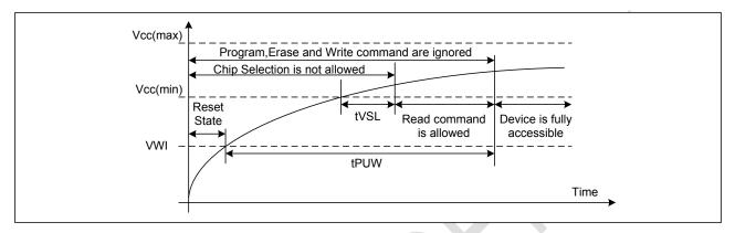
Table3. Power-Up Timing and Write Inhibit Threshold
