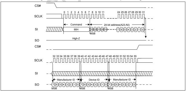
Figure11. Read Manufacture ID/ Device ID Sequence Diagram
