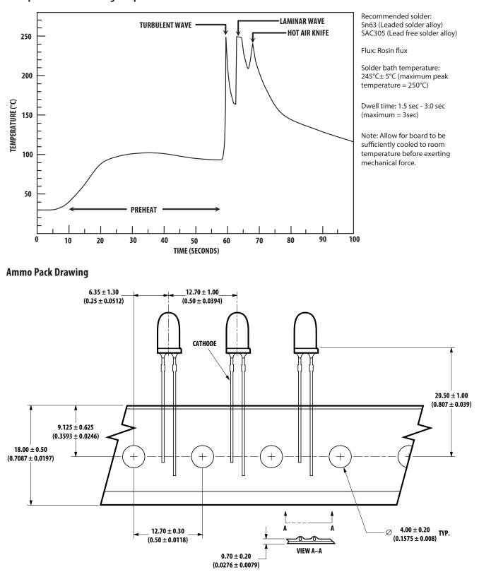
**Example of Wave Soldering Temperature Profile for TH LED**
