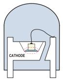
Note: Electrical connection between bottom surface of LED die and the lead frame is achieved through conductive paste.
