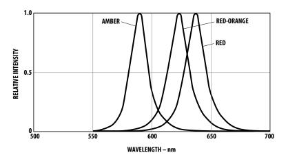
Figure 1. Relative intensity vs. peak wavelength.
