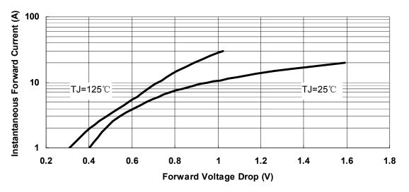
Fig.3-Typical Instantaneous Forward Voltage Characteristics
