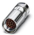
Cable connector, straight, Screw locking, M17, Number of positions: 8, Type of contact: Socket, Crimp connection, shielded: yes, Cable diameter: 5 mm...8 mm
