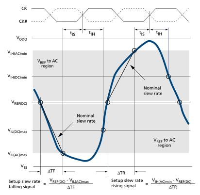
Figure 23: Tangent Line for <sup>t</sup>IS
