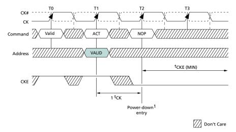
Note: 1. The earliest active power-down entry may occur is at T2, which is 1 × <sup>t</sup>CK after the ACTI-VATE command. Active power-down entry occurs prior to <sup>t</sup>RCD (MIN) being satisfied.
