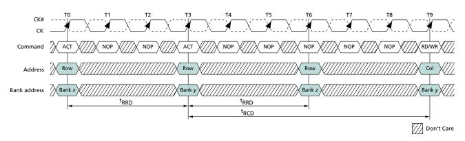
A subsequent ACTIVATE command to a different row in the same bank can only be issued after the previous active row has been closed (precharged). The minimum time interval between successive ACTIVATE commands to the same bank is defined by <sup>t</sup>RC.
