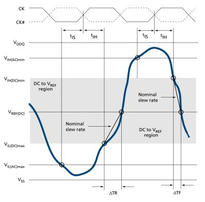
Figure 25: Tangent Line for <sup>t</sup>IH
