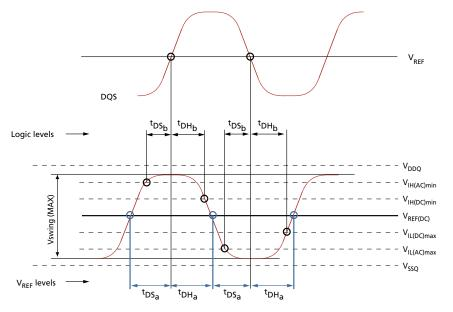
Figure 33: AC Input Test Signal Waveform (Differential)
