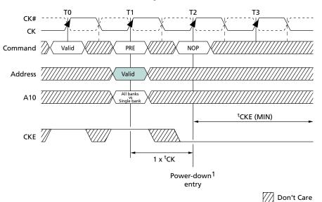
Note: 1. The earliest precharge power-down entry may occur is at T2, which is 1 × <sup>t</sup>CK after the PRECHARGE command. Precharge power-down entry occurs prior to <sup>t</sup>RP (MIN) being satisfied.
