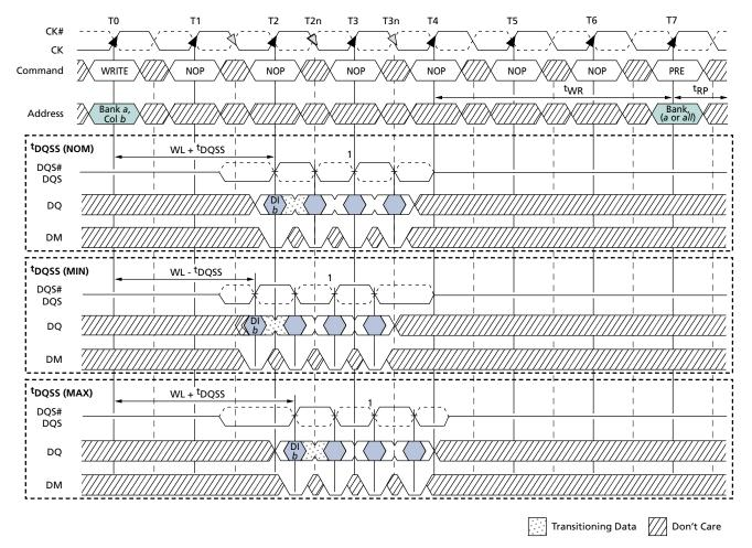
Notes: 1. Subsequent rising DQS signals must align to the clock within <sup>t</sup>DQSS.
