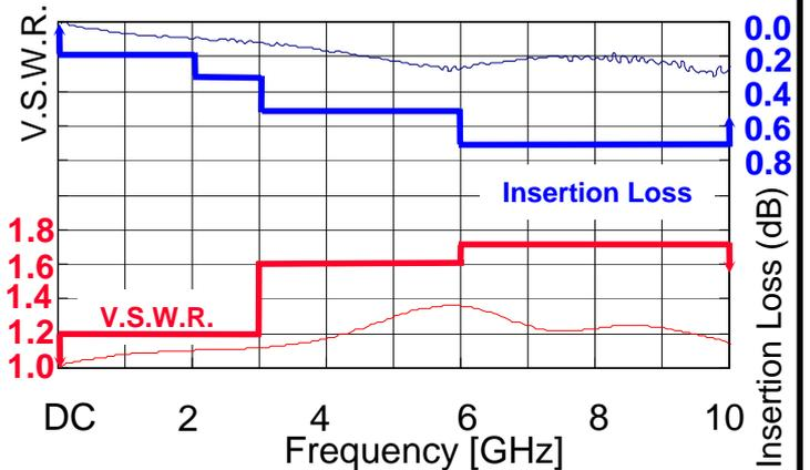
\*\*Tested in the mated condition with MS-162-HRMJ-1.
