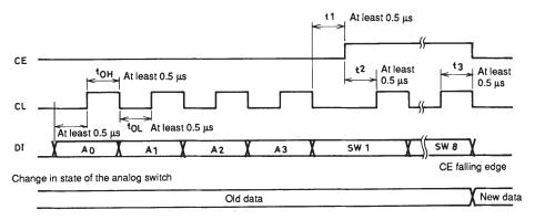
Data is read in on the rising edge of CL and latched on the falling edge of CE.
