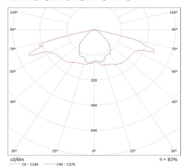
Luminaire: LEDiL Oy C14121\_STRADA-SQ-FS2-NP\_(XHP70)\_glass Lamps: 1 x Cree\_XHP70\_glass-chassis\_260.488lm@250mA\_P=1.38405W\_l=0.2499A
