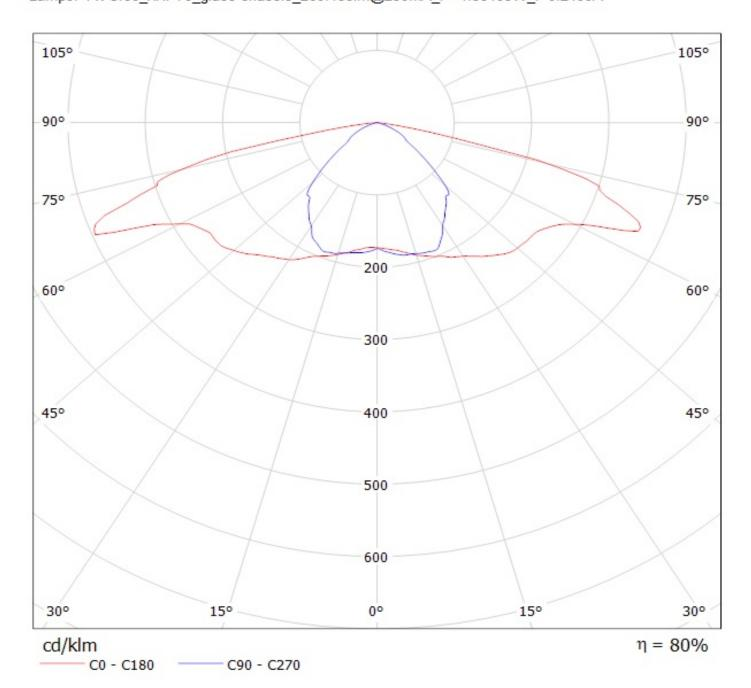
Luminaire: LEDiL Oy STRADA-SQ-FS2 & STRADA-SQ-FS2-NP\_(LUXEON\_M)\_glass Lamps: 1 x LUXEON\_M\_(LXR7-SW30)\_375lm@250mA\_P=2.79W\_l=249.8mA
