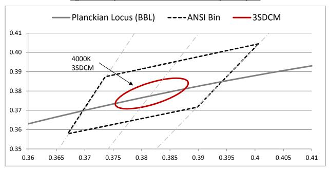
Note: 3SDCM bin is shown inside standard ANSI bins for comparison purposes. Color characteristics specified at  $T_C = 85$ °C.
