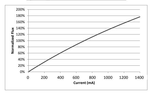
Figure 3: Typical Flux vs. Current – BXRE-xxx-3001-D-xx
