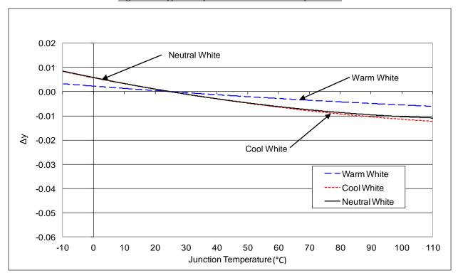
Figure 6: Typical ccx Shift vs. Junction Temperature
