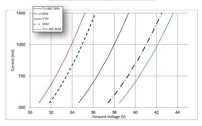
Note:  $T_C$  = 85°C voltage represents minimum voltage at a case temperature of 85°C.  $T_C$ = -40°C voltage represents maximum voltage at  $T_C$ = -40°C.
