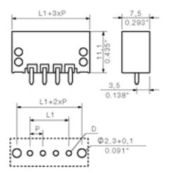
1761142001 SL-SMT3.5/20/180F 1.5SN PCB plug-in connector, Male connectors, Reflow solder connection, Pitch: 3.50 mm, No. of poles: 20, 180°, Box 4032248131716 20 pc(s).
