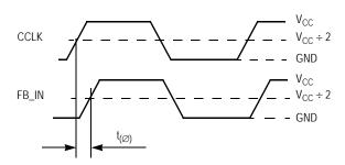
Figure 9. Propagation Delay ( $t_{(\emptyset)}$ , static phase offset) Test Reference
