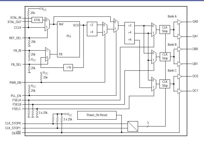
Figure 1. MPC9330 Logic Diagram
