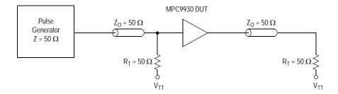
Figure 7. CCLK MPC9330 AC Test Reference for  $V_{cc}$  = 3.3 V
