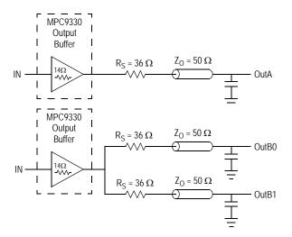
Figure 4. Single versus Dual Transmission Lines
