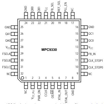
It is recommended to use an external RC filter for the analog power supply pin  $V_{\text{CC\_PLL}}$ . Please see Applications Information section for details.
