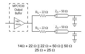
Figure 6. Optimized Dual Line Termination
