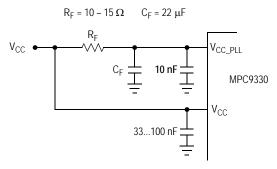
Figure 3.  $V_{CC\ PLL}$  Power Supply Filter
