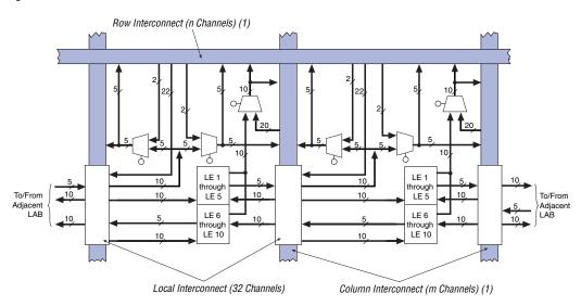
Figure 9. FastTrack Interconnect Architecture
