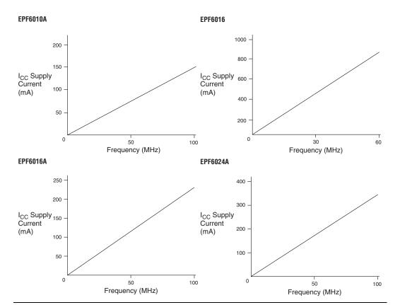
Figure 20. I<sub>CCACTIVE</sub> vs. Operating Frequency
