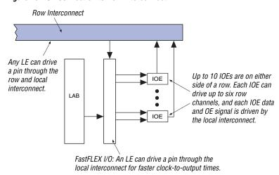
Figure 13. IOE Connection to Row Interconnect
