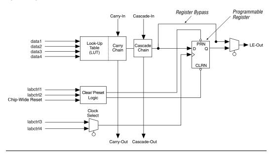
The programmable flipflop in the LE can be configured for D, T, JK, or SR operation. The clock and clear control signals on the flipflop can be driven by global signals, general-purpose I/O pins, or any internal logic. For combinatorial functions, the flipflop is bypassed and the output of the LUT drives the outputs of the LE. The LE output can drive both the local interconnect and the FastTrack Interconnect.
