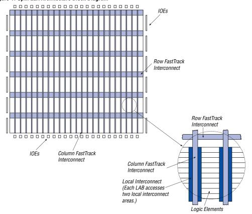
Figure 1. OptiFLEX Architecture Block Diagram
