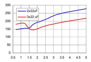
**Note:** Input ripple voltage for various output voltages with  $2x22 \mu F$  or  $3x22 \mu F$  ceramic capacitors at the input (20A load). Input voltage is 12V.
