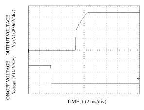
Start-up Using On/Off Voltage (Io = Io,max), Vo=0.69V
