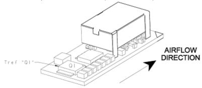
Preferred airflow direction and location of hot-spot of the module (Tref).
