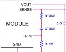
Circuit diagram showing connection of R<sub>TUNE</sub> and C<sub>TUNE</sub> to tune the control loop of the module
