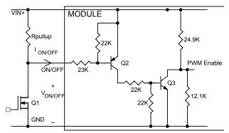
Circuit configuration for using positive On/Off logic
