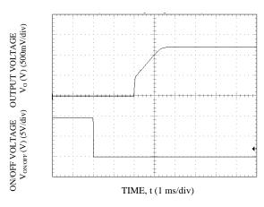
Start-up Using On/Off Voltage (Io = Io,max), Vo=1.2V
