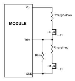
Circuit Configuration for margining Output voltage
