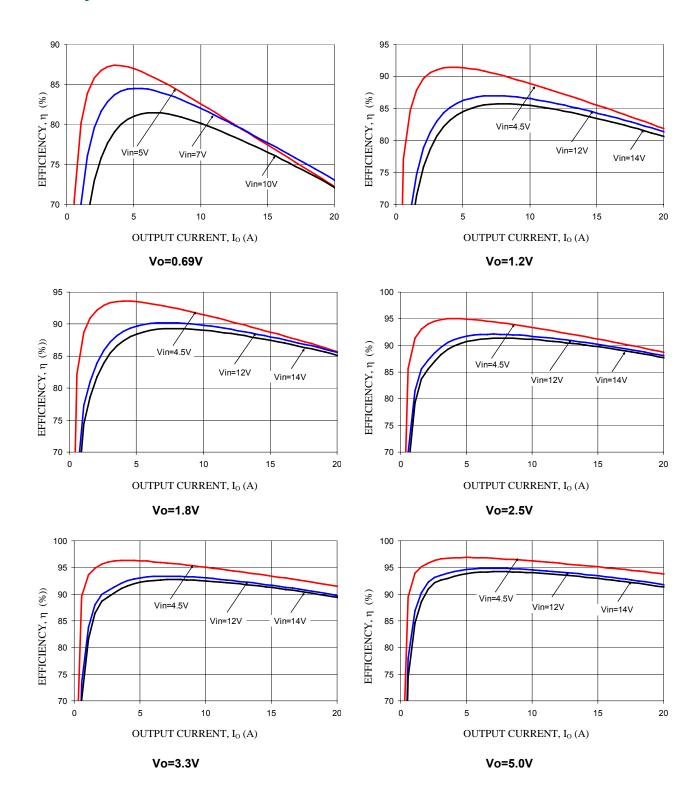
4.5 Vdc - 14 Vdc Input, 0.69 Vdc - 5.5 Vdc /20 A Outputs
