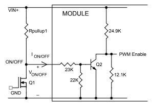
Circuit configuration for using negative On/Off logic
