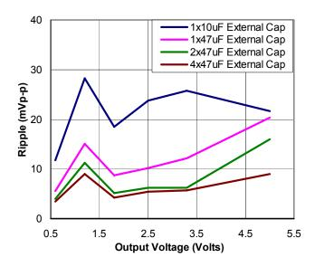
**Note:** Output ripple voltage for various output voltages with external 1x10  $\mu$ F, 1x47  $\mu$ F, 2x47  $\mu$ F or 4x47  $\mu$ F ceramic capacitors at the output (20A load). Input voltage is 12V.
