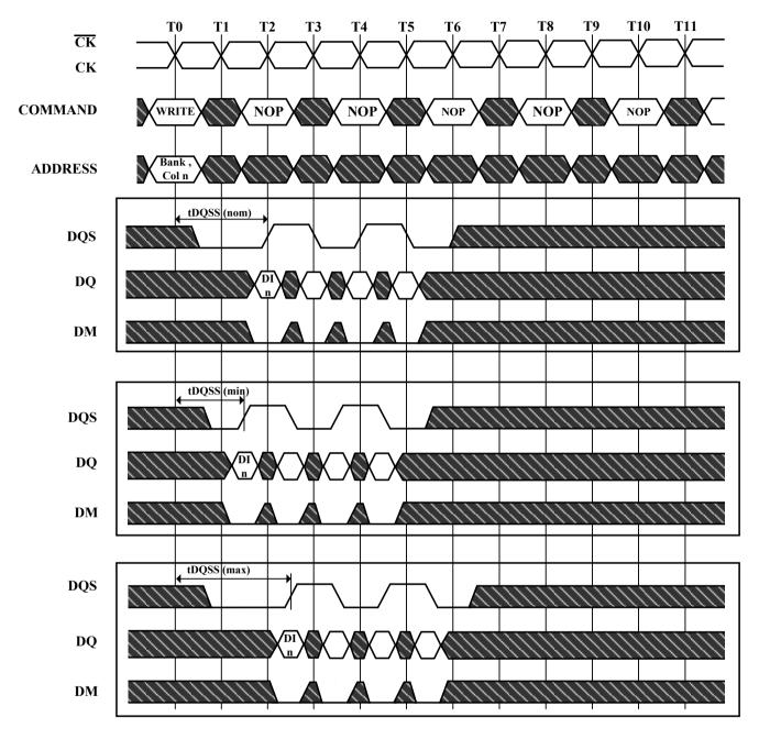
$\boldsymbol{3}$  subsequent elements of Data  $\,$  are applied in the programmed order following DI  $\boldsymbol{n}$
