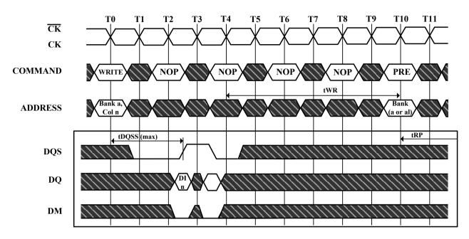
1 subsequent elements of Data In are applied in the programmed order following DI n A non-interrupted burst of 2 is shown
