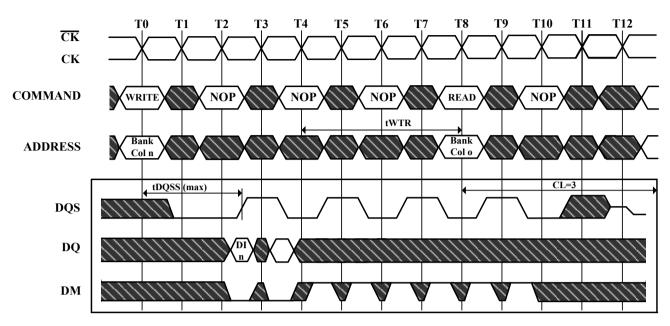
1 subsequent elements of Data In are applied in the programmed order following DI n
