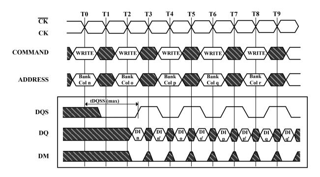
n', etc. = the next Data In following DI n, etc. according to the programmed burst order Programmed Burst Length 2, 4, or 8 in cases shown
