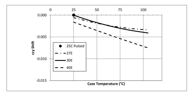
Figure 7: Typical DC ccx Shift vs. Case Temperature
