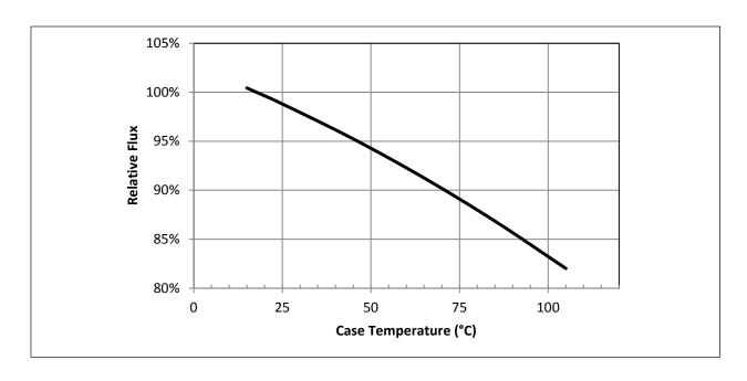
Figure 6: Typical DC ccy Shift vs. Case Temperature
