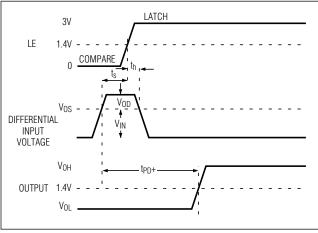
Figure 2. MAX9109 Timing Diagram
