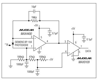
Figure 4. Battery-Operated Infrared Data Link Consumes Only 760µA
